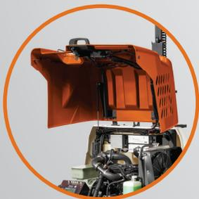
**GAS-ASSISTED REAR HATCH** opens easily, and stays secure for quick and easy unobstructed maintenance access
